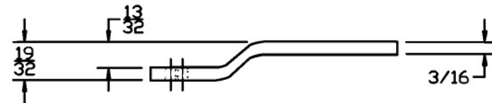
RIGHT REINFORCEMENT SIDE VIEW
